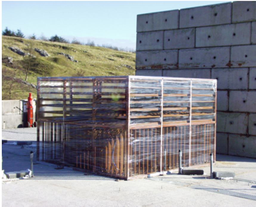
Figure 1. Congestion rig with plastic film in position
