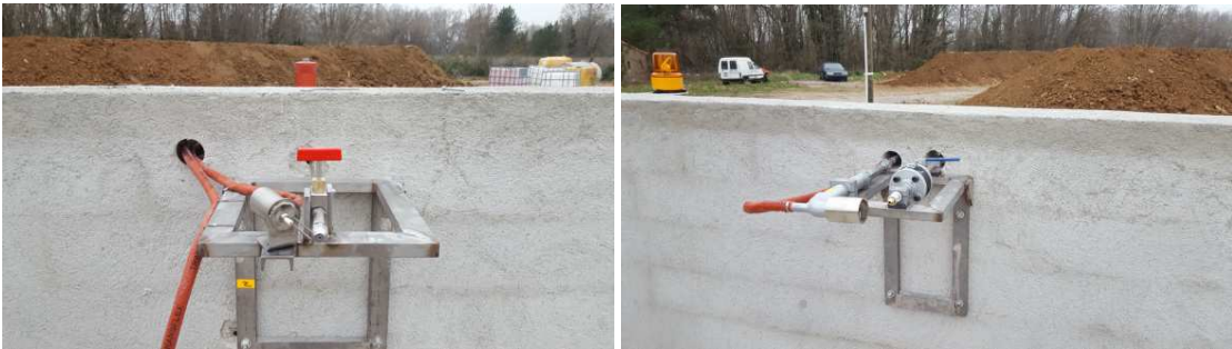
Figure 8. Hydrogen (left) and LPG (right) jet fire release nozzles and their ignition sources.
