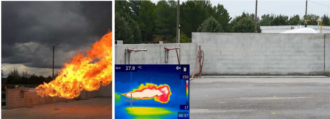
Figure 9. 20 bar LPG (left) and 200 bar hydrogen jet fires (right).
