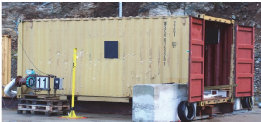
Figure 1: ISO container with displacement sensor and target plate.
