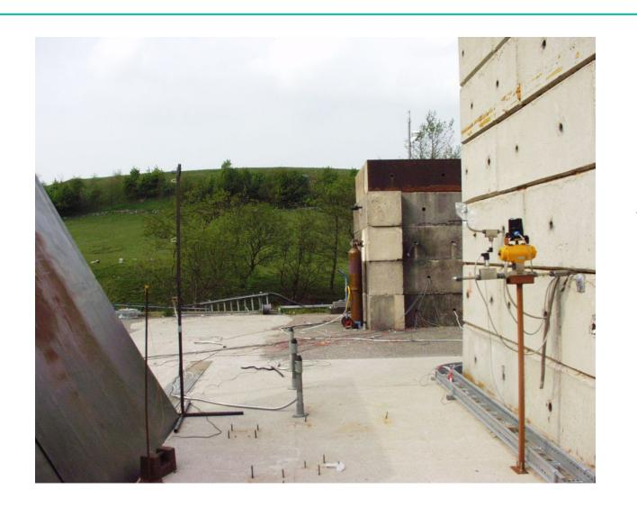
Pressure sensors in front of 60 ° barrier and relative to wall
