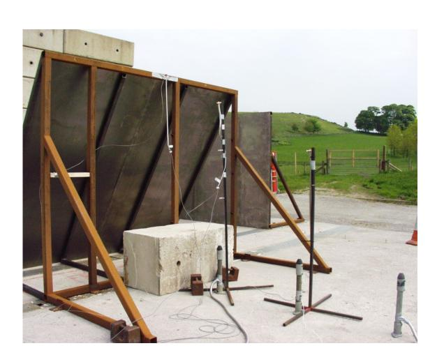
Pressure sensors at back of barrier
