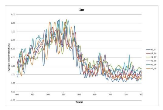
Figure 8. Hydrogen concentration within the enclosure at the 1 m level, 1200 Nl/min, one upper vent, one lower vent, wind blowing into the upper vent
