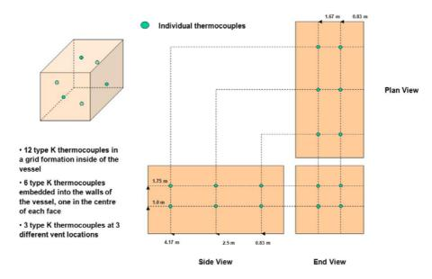
Figure 5. Positions of thermocouples within enclosure
