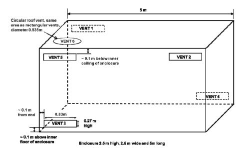
Figure 1. Sketch of the HSL 31 m<sup>3</sup> test facility
