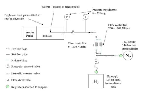
Figure 2. Schematic of the Hydrogen supply system
