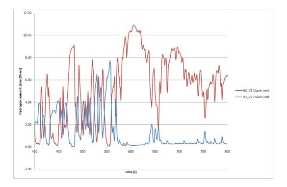
Figure 9. Hydrogen concentration at the upper and lower vents, 1200 Nl/min, one upper vent, one lower vent, wind blowing into the upper vent
