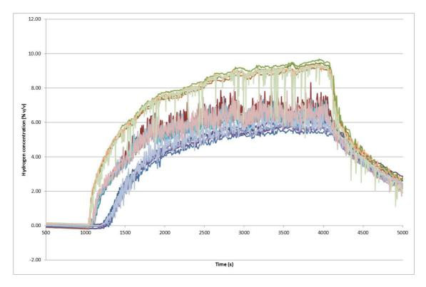
Figure 6. Hydrogen concentrations within the enclosure, 150 Nl/min single upper vent, minimal influence of wind
