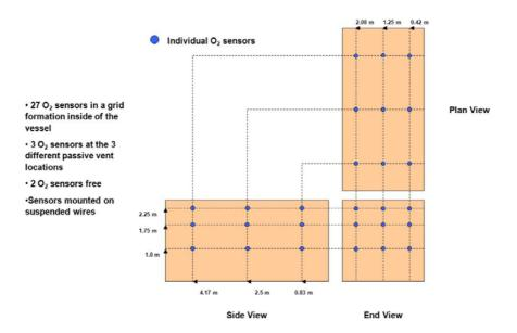
Figure 4. Positions of oxygen detectors within enclosure (for hydrogen concentration measurements)
