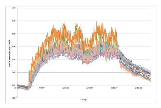
Figure 7. Hydrogen concentrations within the enclosure, 150 Nl/min single upper vent, marked influence of wind blowing into open vent
