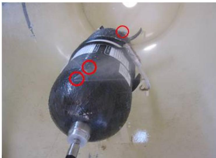
Figure 3. Leakage of Type -3 Cylinder
