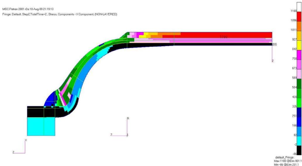
Figure 6. Stresses and Strains at Max. Fill Pressure
