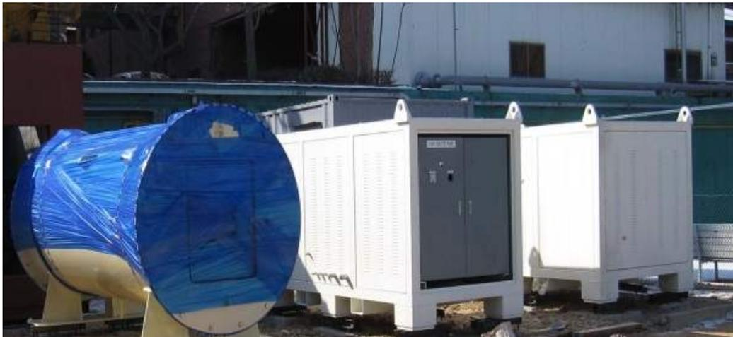
Figure 1. High Pressure Pump and Chamber
