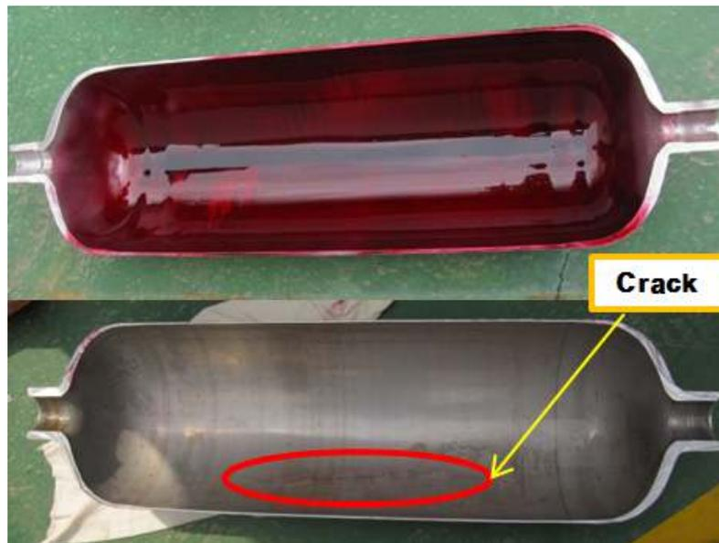
Figure 4. Penetration Test for Inner Liner of Type-3 Cylinder
