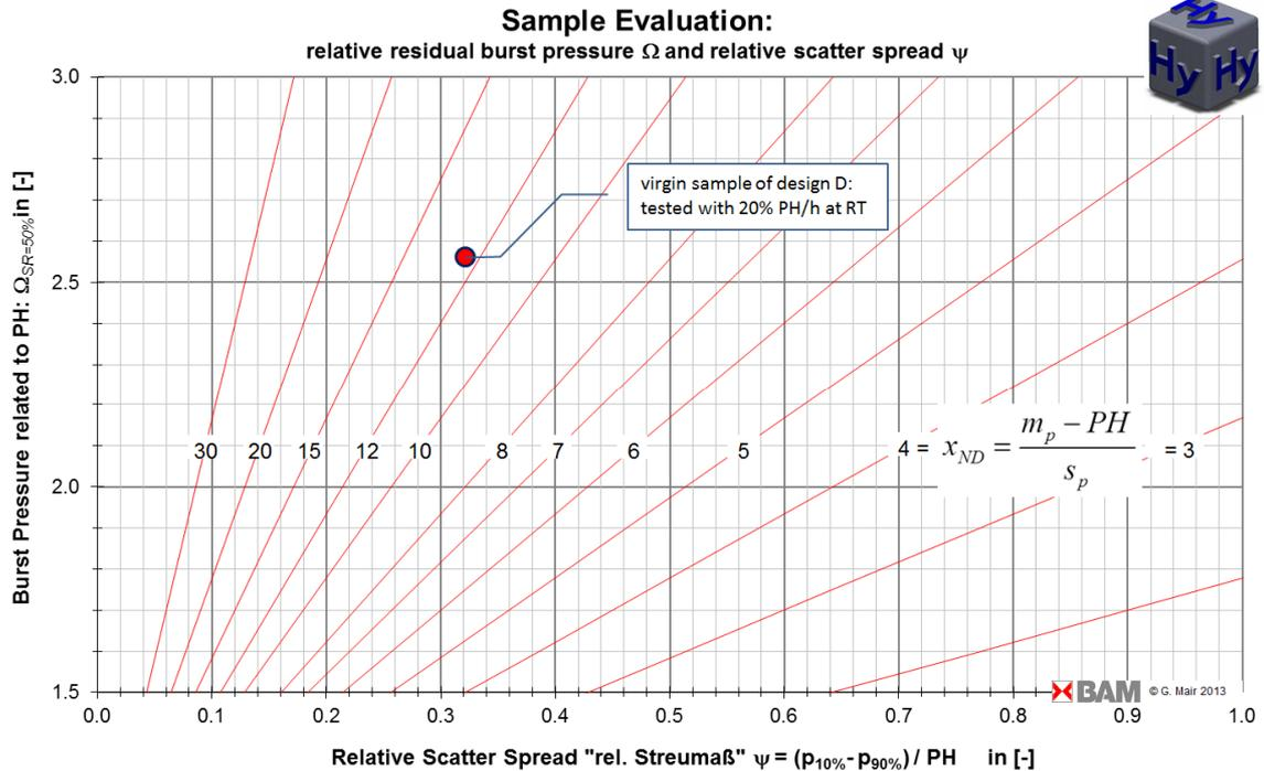
Figure 4: Result of evaluation of the slow burst tested sample of virgin specimens of design D
