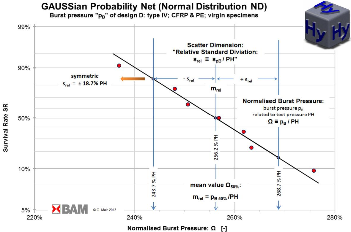
Figure 2: Results of Fig 1 after normalisation of data (Division by test pressure PH)
