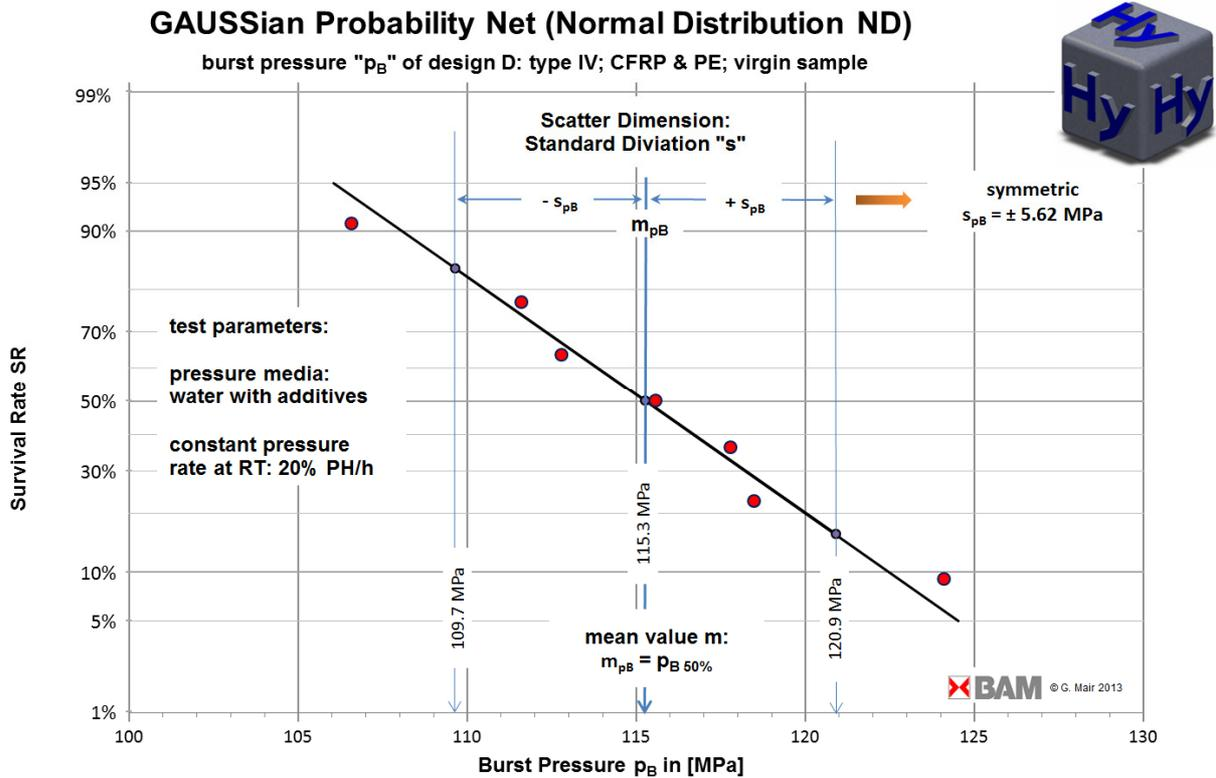
Figure 1: Plot of individual test results, mean value and standard deviation from Table 1
