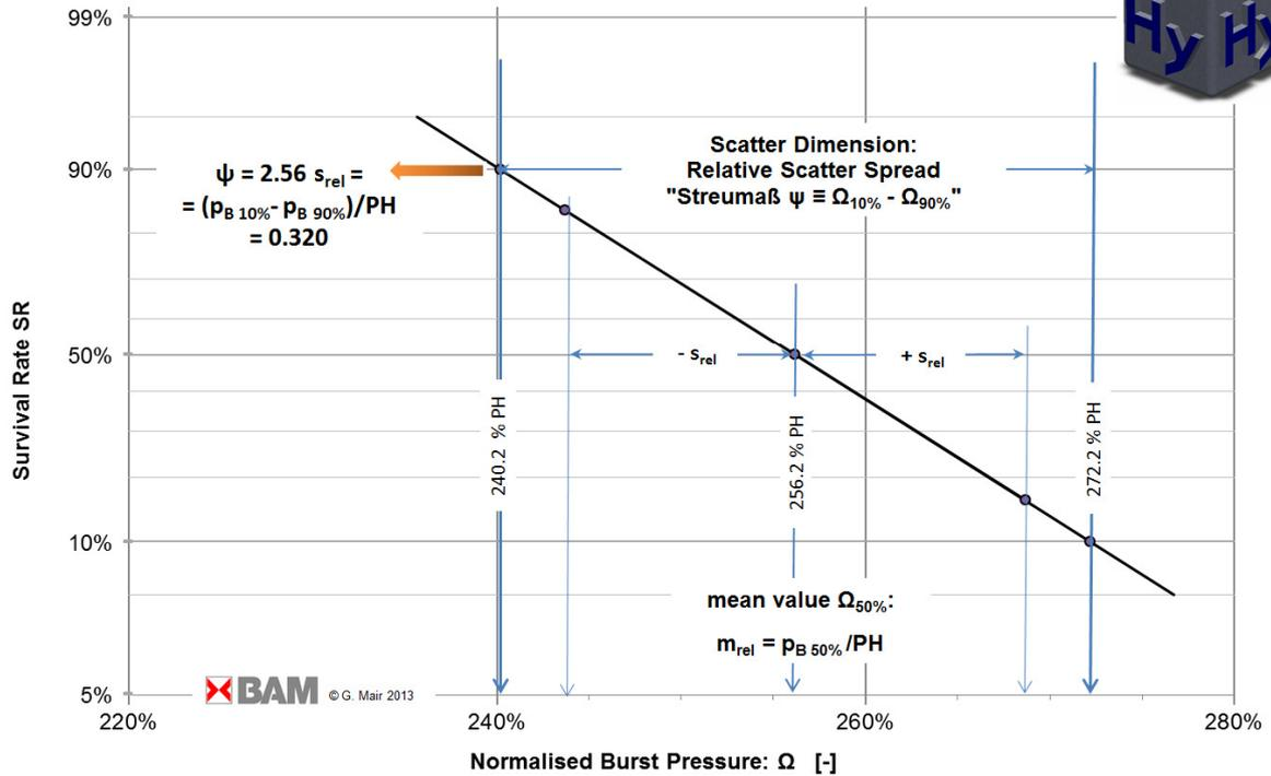
Figure 3: Values of Fig 2 by using "Streumaß" for quantification of relative scatter
