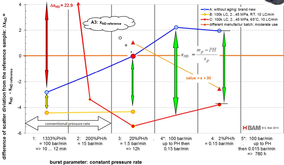
Figure 8: Normalised deviation rate as indicator of reliability over pressure rate
