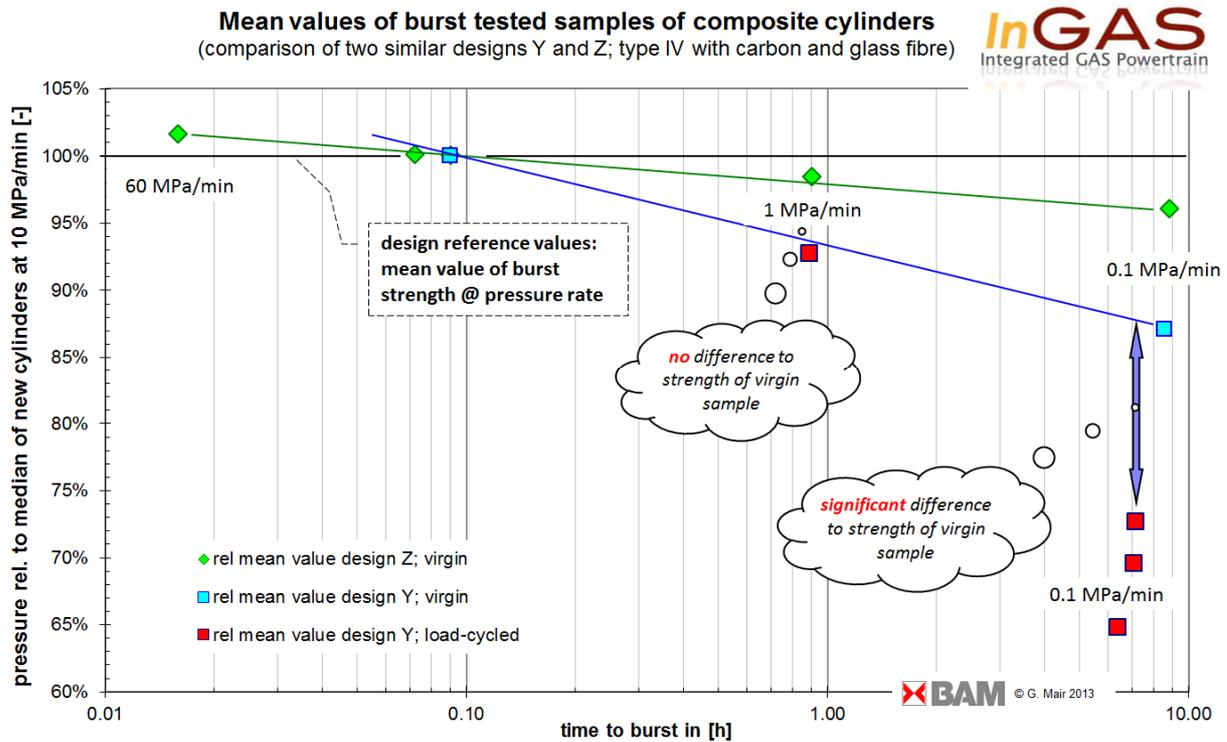
Figure 1: Influence of pressure rate on burst pressure: GFRP/CFRP-design types with plastic liner
