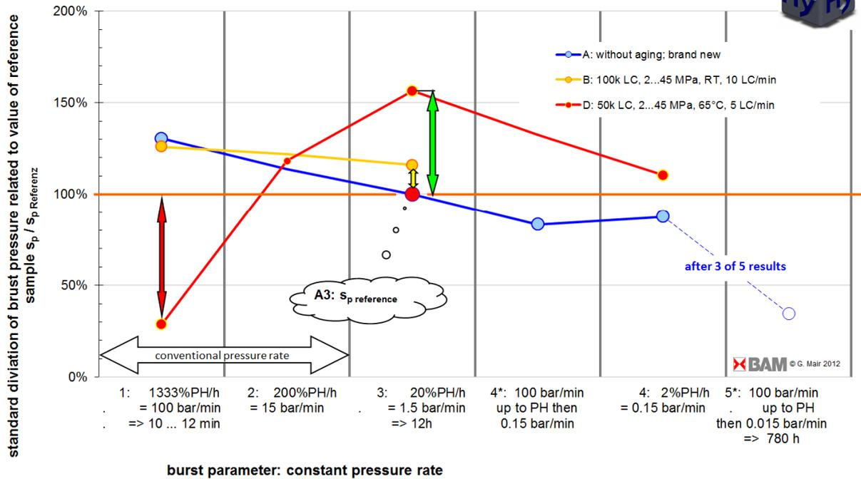
Figure 7: Standard deviation over pressure rate
