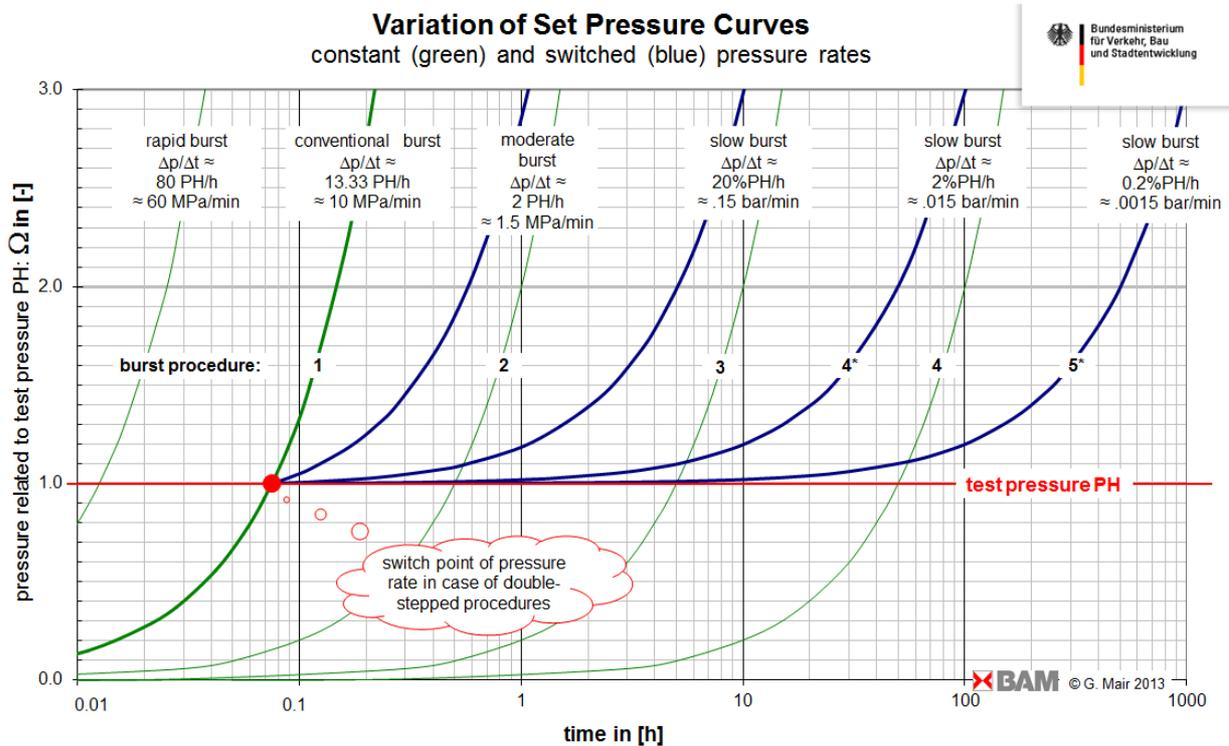
Figure 2: Representation of different pressure-time curves as a test parameter
