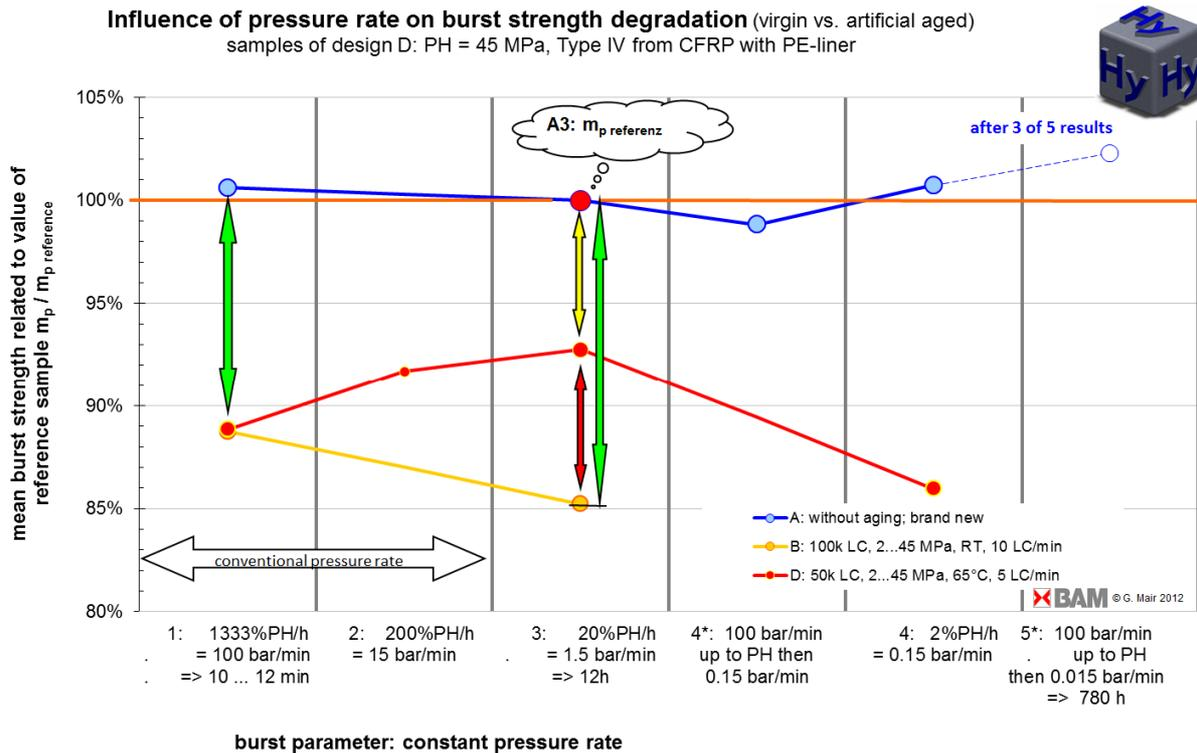
Figure 6: Mean values of burst pressures over pressure rate
