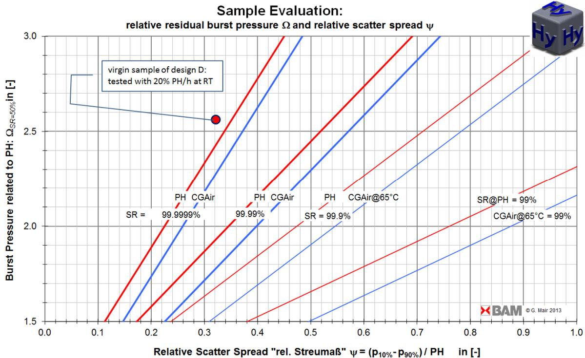
Figure 5: Comparison of tested sample properties with lines of reliability
